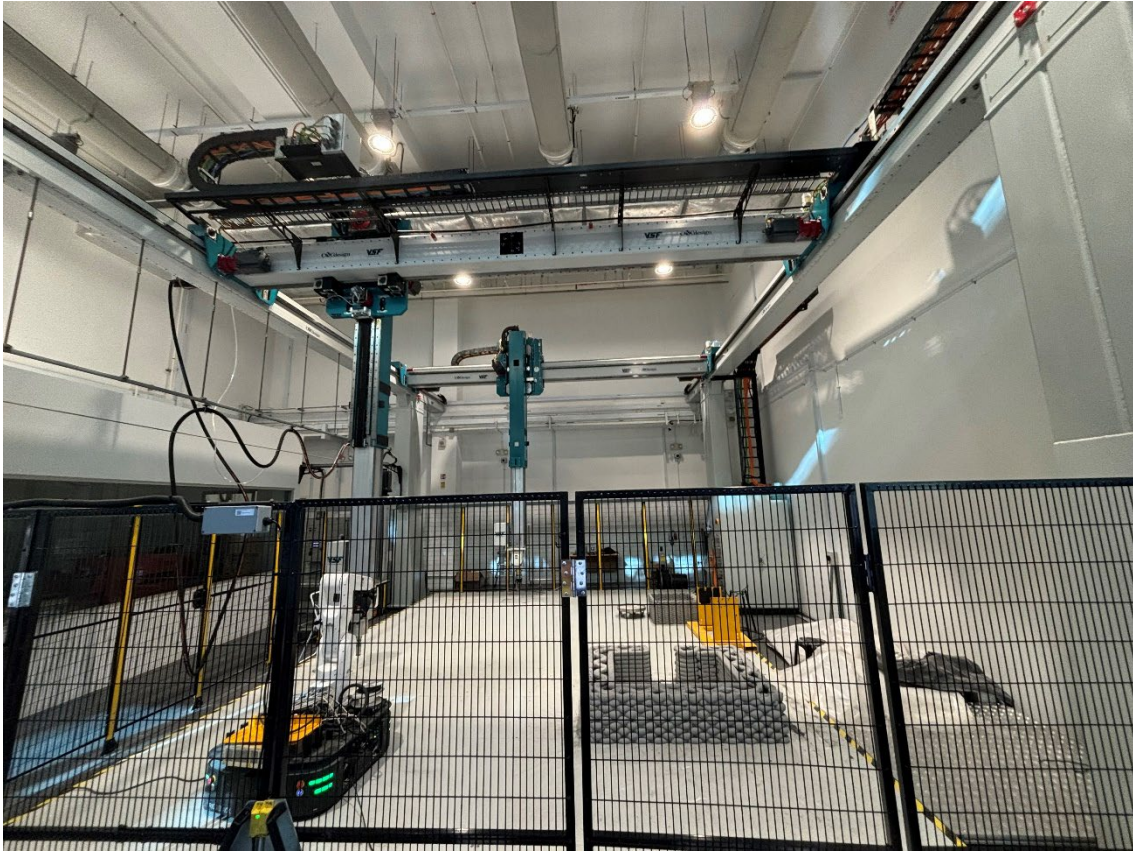
3D Printer for Printing with Concrete
