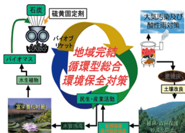
◎Fig. 15. An Example as zero-emission cycle using bio-briquetting of raw coal.
