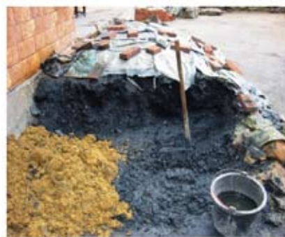
Fig. 7. Mixed fuel prepared from raw-coal and clay.
