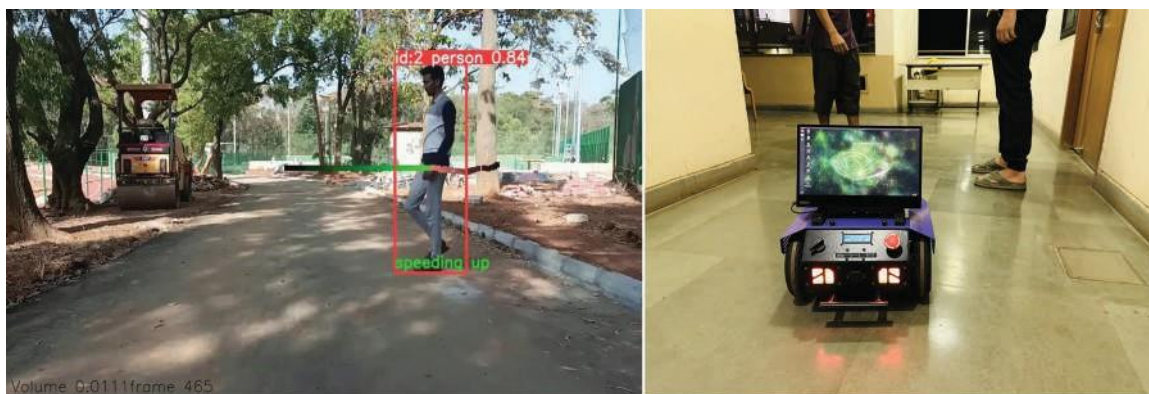
(a) Identification of pedestrians from monocular camera images (b) YATI, the robot used for experiments
